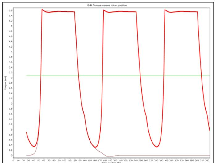
Figure 6 Torque ripple of the VSR motor.
