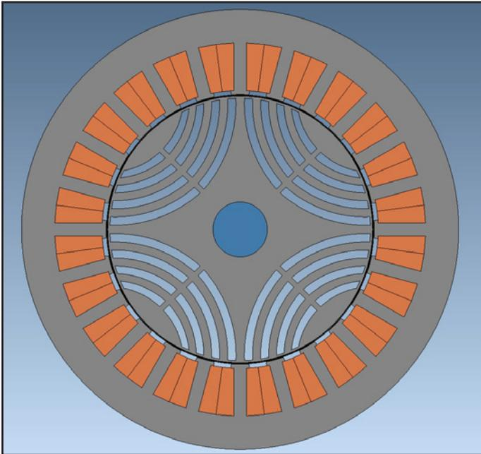
Figure 7 Lamination of the SYR motor.
