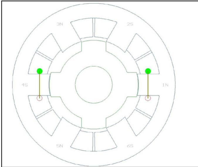
Figure 1 Basic lamination design of a VSR motor.
