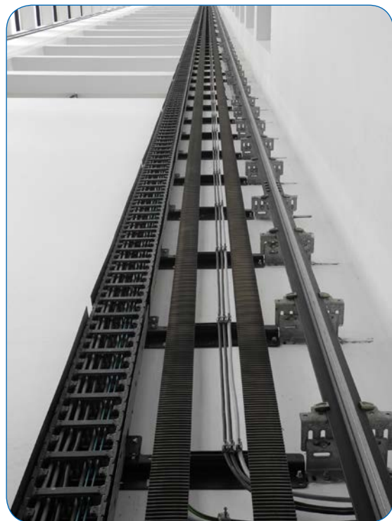
For the project in Singapore, Wöhr ordered 6,600 feet of the timing belt Conti Synchrondrive (photos courtesy of ContiTech).
