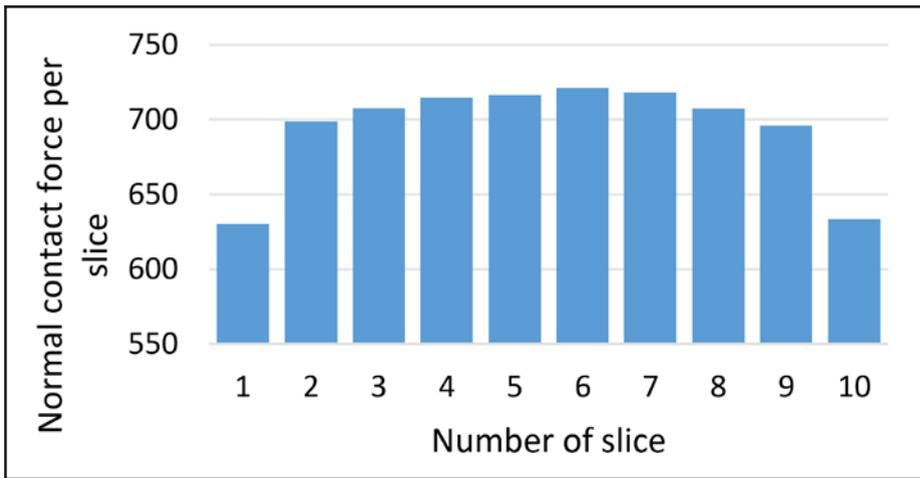
Figure 5 Contact normal forces distribution in cylinder.
