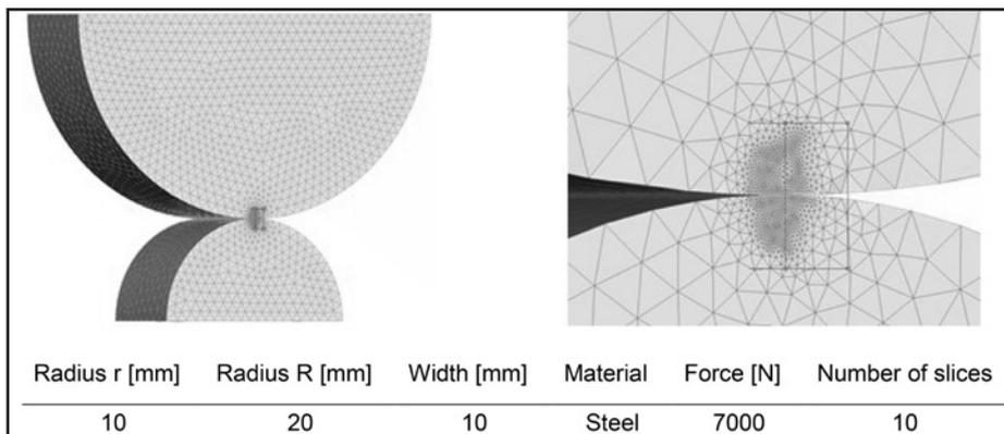
Figure 4 Hertzian contact model data and mesh.
