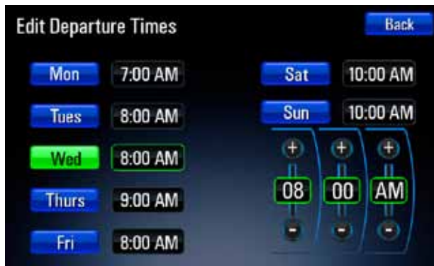
2011 Chevrolet Volt Delayed Charging Screen - The 2011 Chevrolet Volt allows owners to program charging times based on departure time from the Volt's center stack 7-inch LCD touch screen.
