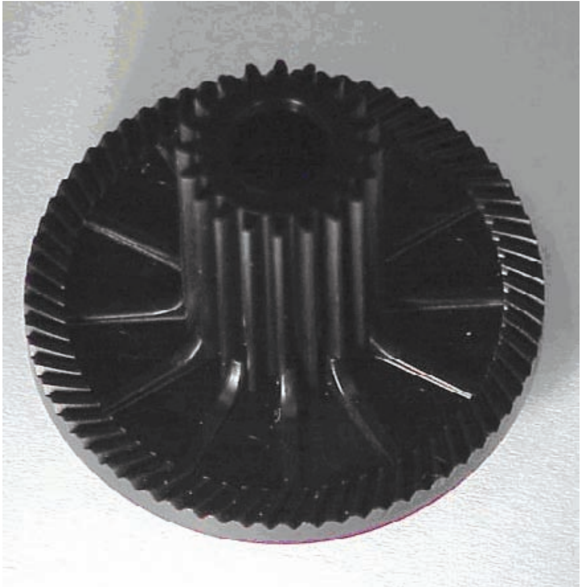
Figure 14—A 30.5° helical angle on pinion printer application: 0.5 module, 69:11 ratio helical face gear with a 90° shaft angle.
