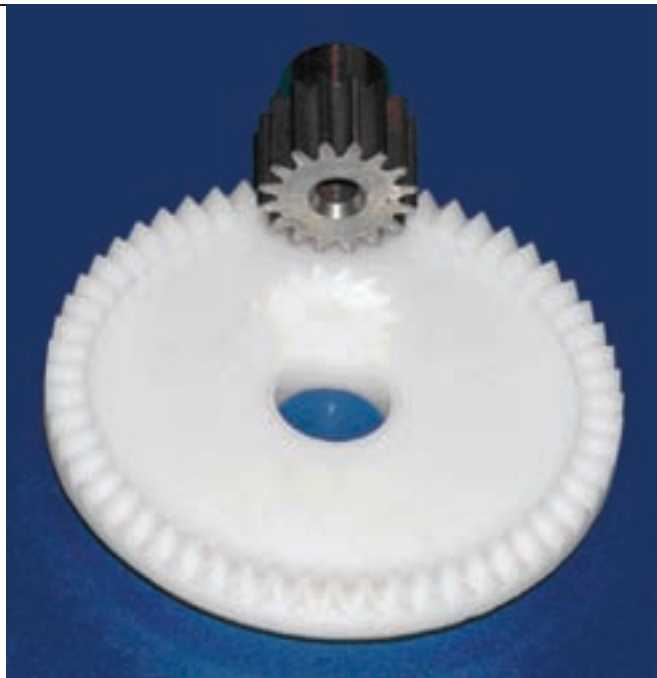
Figure 2—A 90° shaft angle wheelchair access door opener application: 20 diametral pitch, 56:16 ratio.
