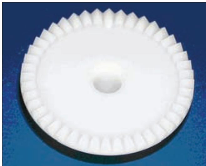
Figure 1—Power tool application: 28 diametral pitch, 44:15 ratio face gear, 90° shaft angle.
