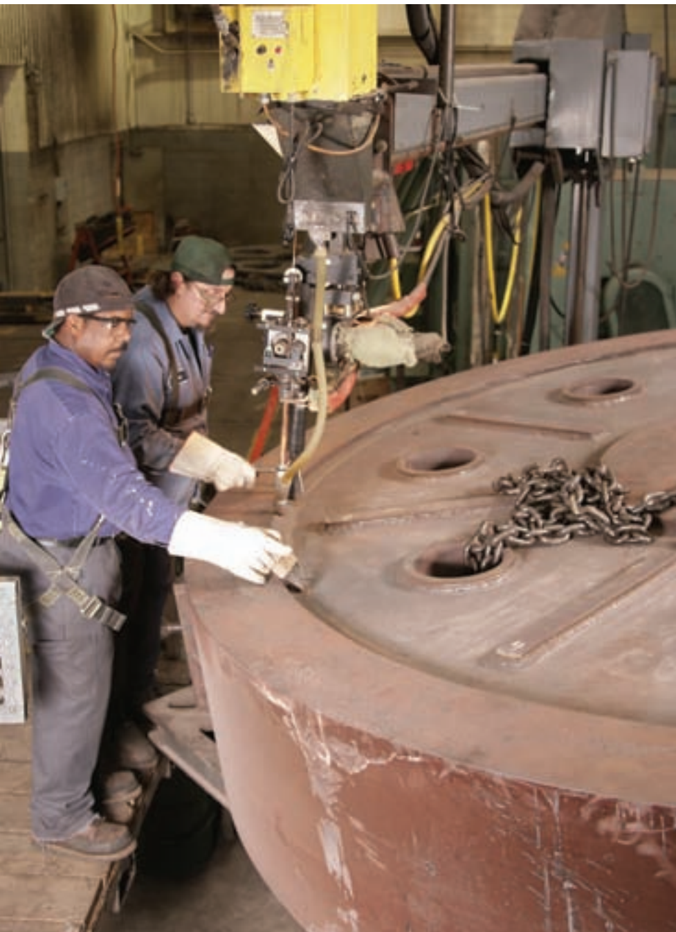
Horsburgh & Scott welders Barry McDowell (front) and Dave Evans (back) create fabricated gears from three components—the outer ring, from which the gear teeth are cut; the inner hub; and the internal webbing that acts as the spokes of the wheel.
