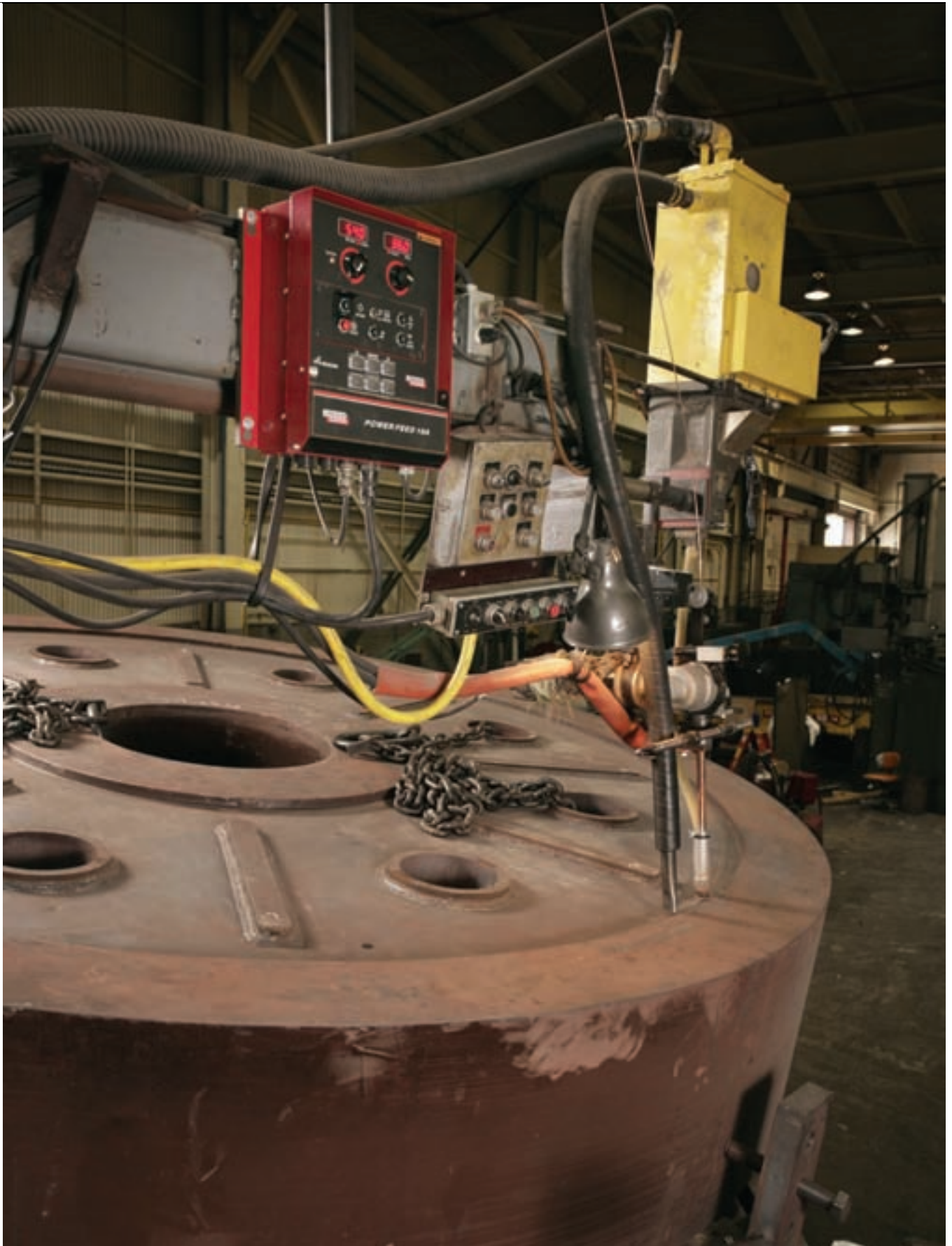
Horsburgh & Scott uses Lincoln Electric's Power Wave AC/DC 1000 power source with Power Feed 10A for submerged arc welding.
