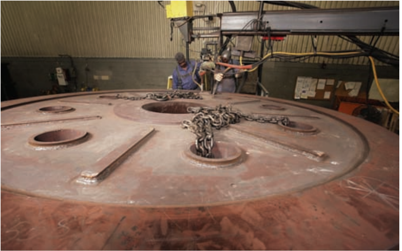
Barry McDowell (left) and Dave Evans (right) welding one of Horsburgh & Scott's gears. When finished, these massive gear blanks can weigh 60 tons and have diameters of 20 feet.
