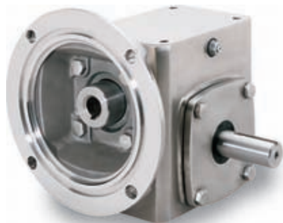
The Boston Gear 700 Series "all stainless steel" worm gear speed reducer is specifically designed to operate in the food industry. Boston Gear uses Klübersynth UH1-6-460 oil to comply with sanitation and health guidelines when operating within the food zone.
